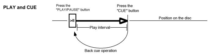
Pressing the "PLAY/PAUSE" button starts the disc. Pressing the "CUE" button will reset the disc to the last place where the disc was started. This is called the cue point. By alternately pressing the "PLAY/PAUSE" button and the "CUE" button, the disc may be returned and played from the cue point any number of times. This function is called back cue.
